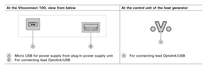
1. Use the Optolink/USB connecting cable to connect the Vitoconnect 100 to the heat generator.
